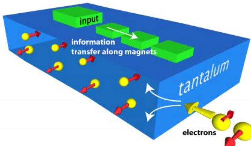
As the current passes through a strip of tantalum, electrons with opposite spins separate. This “clocking” helps in orienting nanomagnets (on the top of the tantalum strip) so that they can be switched easily. New work by University of California Berkeley researchers could one day make nanomagnetic switches a viable replacement for the conventional power-consuming transistors found in all computers.
